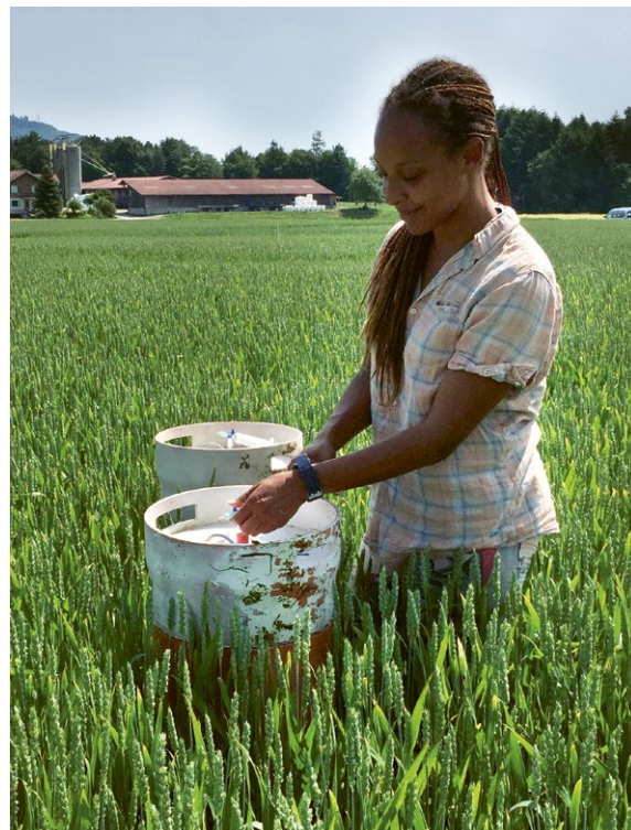
Trapping greenhouse gasses in gas tight chambers installed in a wheat field. GHG gas accumulation in the chambers is measured by taking several gas samples consecutively. These are brought to the lab, where they are analysed by gas chromatography.
