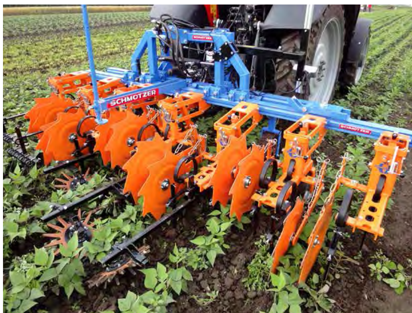
Whereas in arable crops mainly the harrow is used, sophisticated hoeing equipment is employed in vegetable production.
