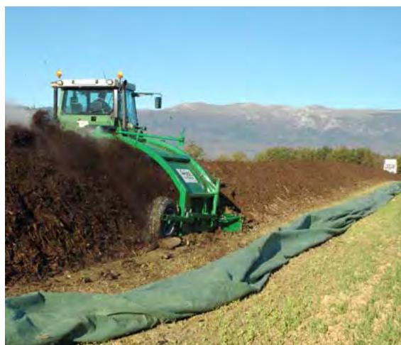
Manure and green waste can be turned into valuable compost in a controlled rotting process at the edge of fields along pathways.
