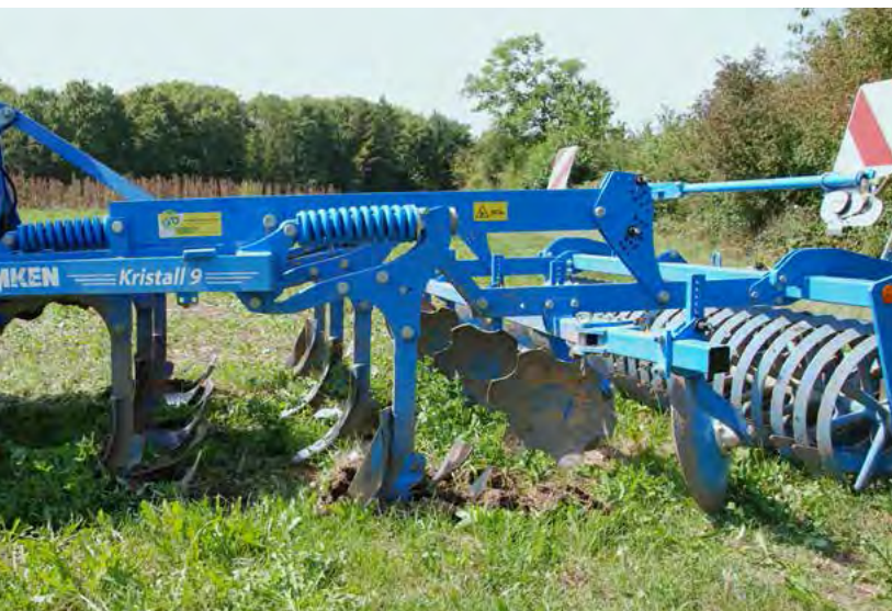
This flat cultivator undercuts the crop with overlapping goosefoot shares over the entire surface and only minimally mixes the soil. This soil-friendly implement combination is particularly suitable for basic soil cultivation on fields with few weeds after crops with little crop residue (e.g. between two cereal crops).
