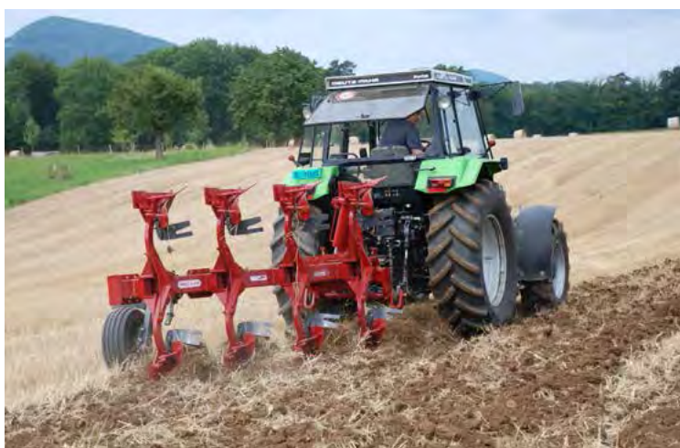
The skim plough is the simplest form of gentle soil cultivation.
