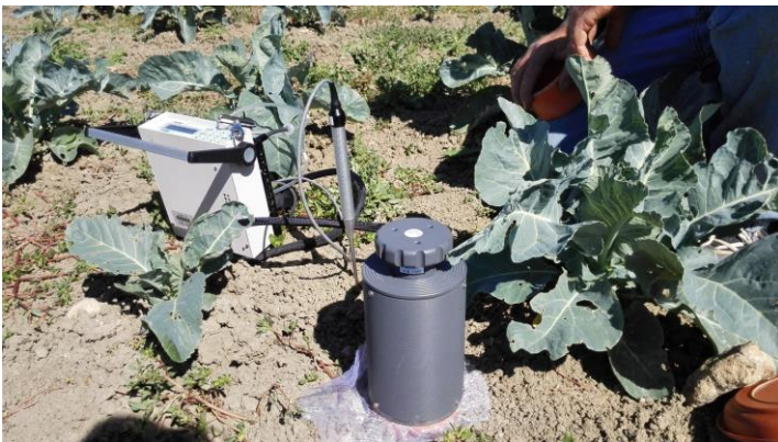
Figura 6. Soil respiration chamber (portatile) PP-System SRC1-EGM4
