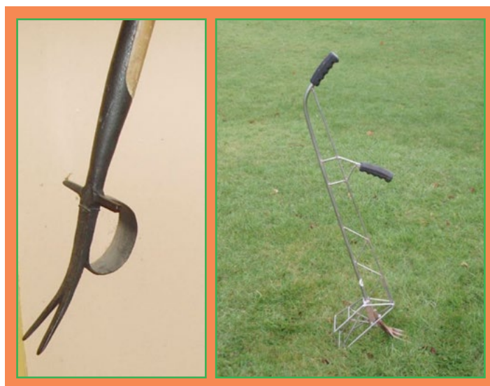
Picture A5. Traditional dock fork (left), modern ergonomic design with interchangeable heads (right)
