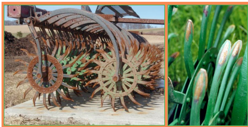
Picture 3. Rotary hoe or spoon weeder
