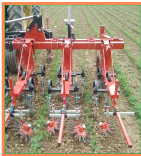
Picture 6. Parallelogram inter-row hoe
