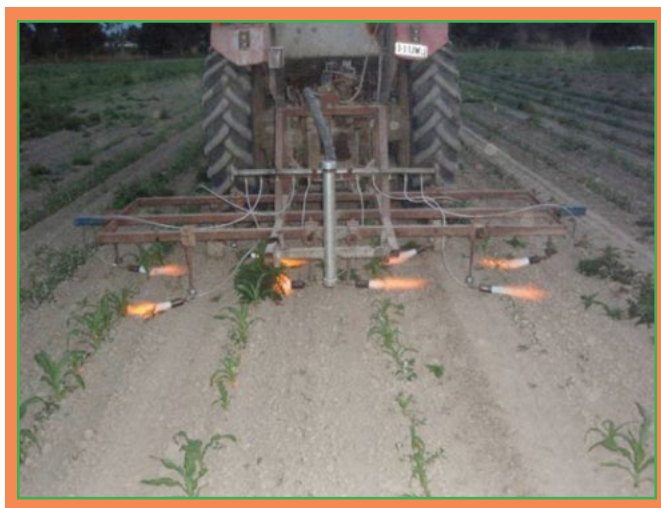
Picture 15. Selective, intrarow flame weeder working in sweetcorn
