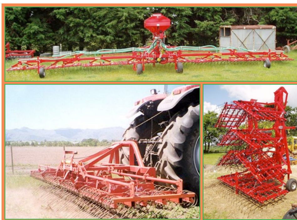
Picture 2. Spring tine weeder.
