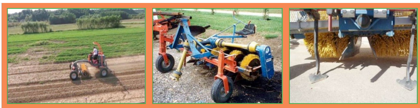
Picture 9. Horizontal axis brush hoe
