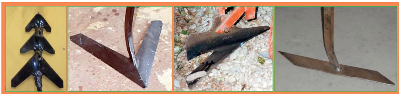
Picture 7. Inter-row hoe blades. Left to right: duck or goose foot, A blade sweep, L blade hoe, T hoe
