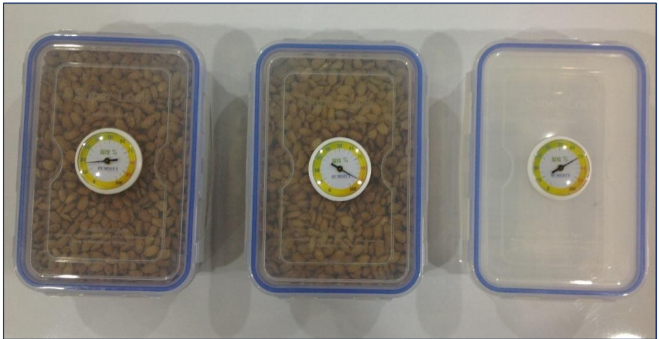
Figure 2: An example of measuring relative humidity of 2 wheat samples. Once they have reached an equilibrium, the one on the left is at about 20% RH and safe for storage. The one in the middle is at about 90% and requires drying. Photo: S. Groot.
