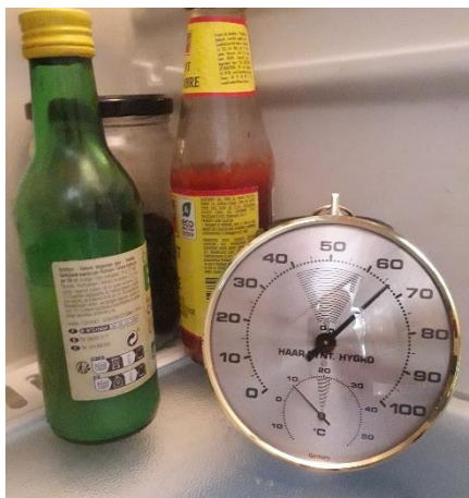
Figure 3: In this refrigerator, relative humidity is at about 65% - too high for seed storage in permeable bags.
